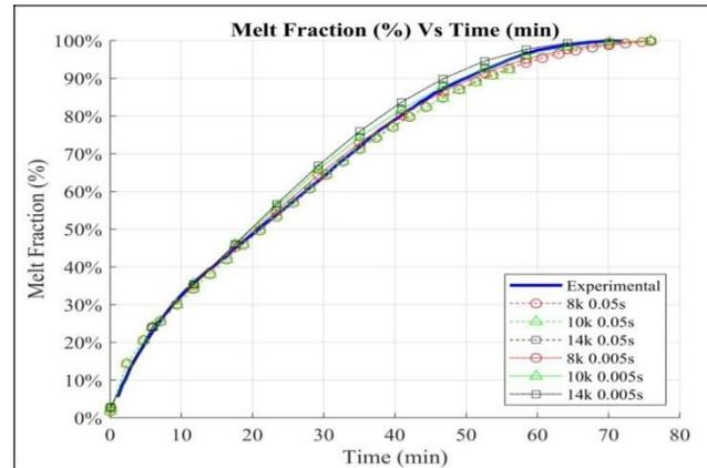
Figure 15: Mesh and Time sensitivity for C = 106 from 0.05s to 0.005s
