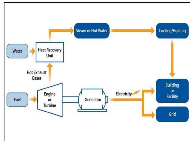
Figure 1: CHP Process Flow Diagram
