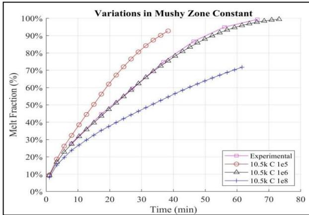
Figure 4: Melt Fraction Vs Time (min)
