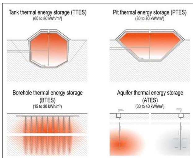
Figure 2: Types of Large-Scale Sensible thermal storage systems
