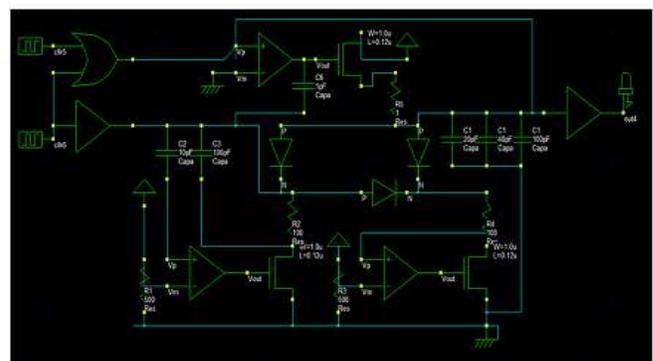
**Fig.4. Circuit diagram of the OLED buffer**
