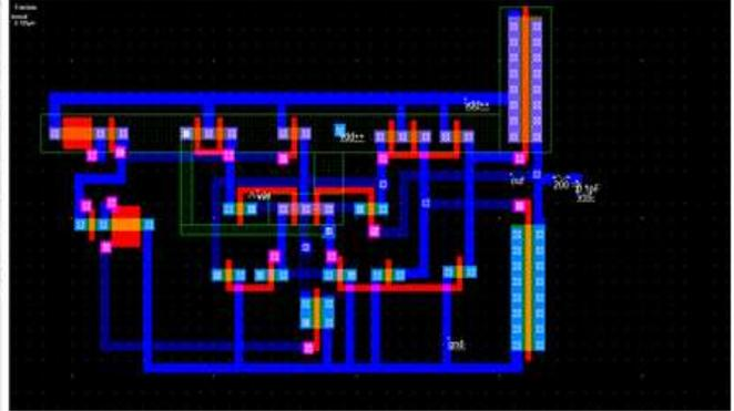
Fig.7. Layout of the implemented buffer
